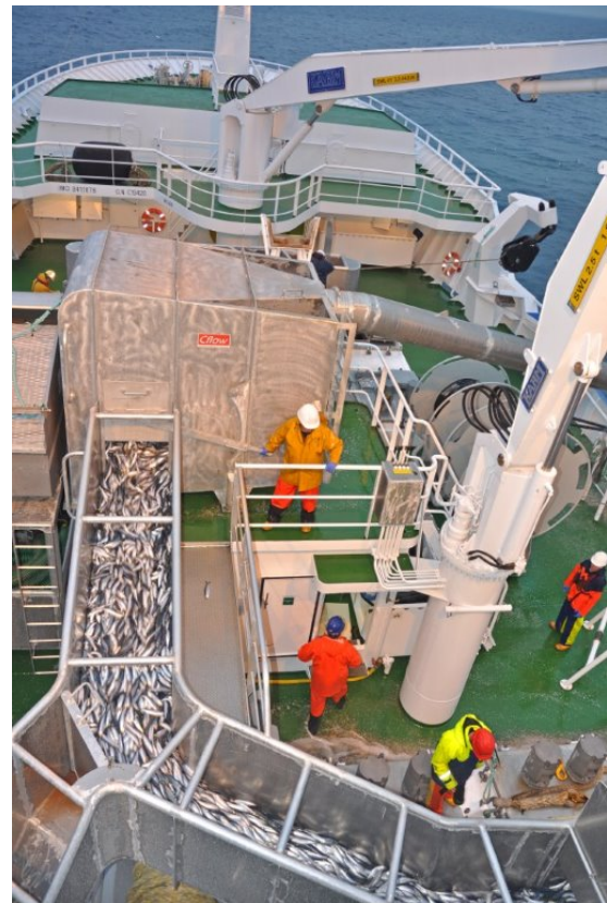
Figure 5. A catch being pumped through the 'separator' to the RSW tanks
