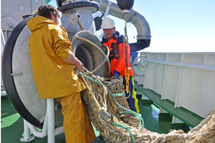
Figure 3. Net being attached to fish pump
